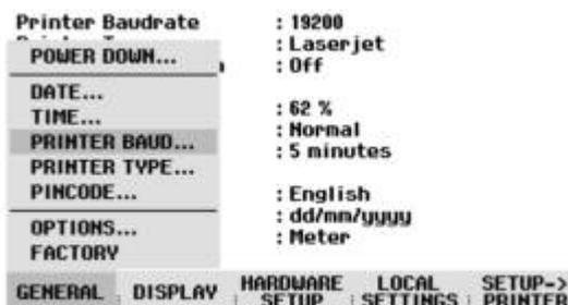
The selection box for the available baud rates (1200 baud to 115 200 baud) opens.
