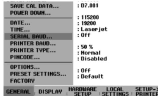
The selection box for the available baud rates (9600 baud to 115200 baud) opens.
