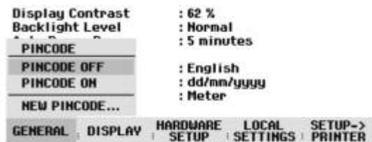
The current PIN must be entered before it can be modified. This prevents unauthorized PIN modification.
