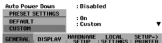
The parameters defined in the data set for the default setup are now used as the preset settings. If no user-specific default setup is defined, CUSTOM is inactive and cannot be selected. The data set defined as the user default setup can be viewed using the R&S FSH3-TV's recall function.
