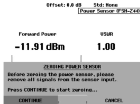
The R&S FSH3-TV immediately starts power sensor zeroing. While this is being done, the R&S FSH3-TV outputs the message "Zeroing power sensor, please wait...".
