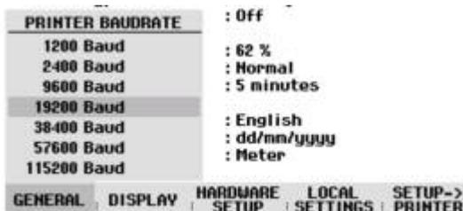
*Note: If the serial/parallel converter (R&S FSH-Z22) is used to control a printer with a parallel interface, set the RS-232-C interface to 38 400 baud.*
