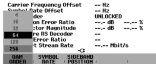
*Note: With J.83/B 64QAM, the R&S FSH3-TV sets the symbol rate to 5.056941 MHz and the roll-off factor to 0.18.*
